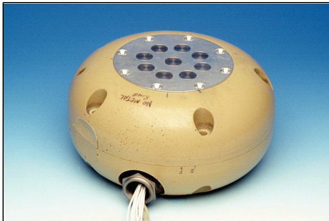
Pressure Footprint Instrumentation Used in Land Mine Neutralization Tests
