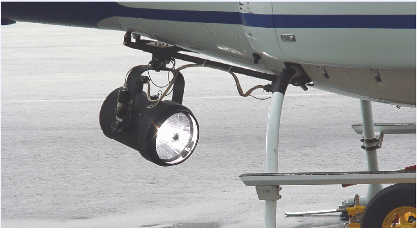
SX-16 NightSun Installed on AS350 Helicopter With Amtech's Mount (FAA and Transport Canada Approved)
